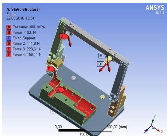
Fig. 3.- Static structural loads, modeling of the load performing
