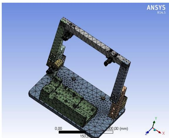
Fig. 2. – Discretization of the geometry model
