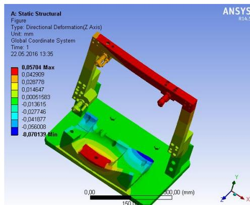
Fig. 7.- Directional Deformation- Z axis
